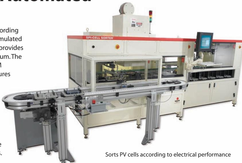
Sorts PV cells according to electrical performance
