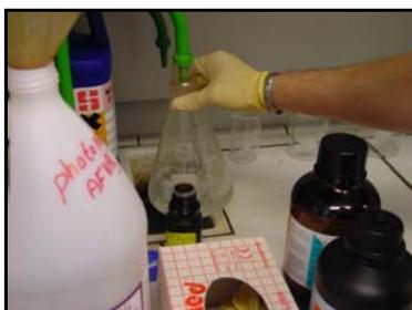
12) When all required solution has been prepared, thoroughly clean all used glassware and the stirring magnet with DI-water. A small amount of DI-water should be left in the Erlenmeyer flask.
