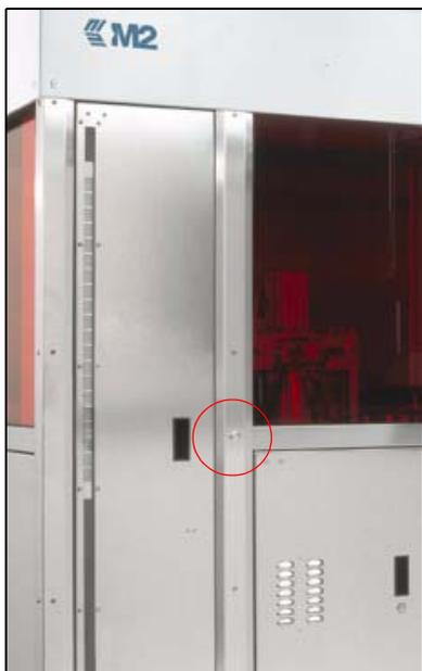
The door to the Stack module is fitted within an interlock device that prevents the door from being opened until the stack lift mechanism has been moved to the default position and has fully stopped. Movement of the stack lift mechanism to the safe default position is activated using the push button located next to the Stack module door.
