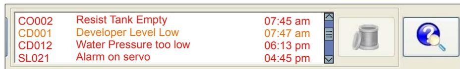
The messages are categorised as either warnings (**Orange Text**), during which the module continues processing, or as errors (**Red text**) which result in production in the module being suspended until rectification of the error.
