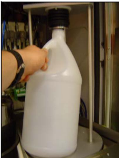
The requirement for emptying of the photo-resist waste vessel is provided by the display of an alarm message at the HMI. The waste bottle is fitted into a neck holder that has as shut-off valve to prevent drips and fumes. Remove the waste bottle by tilting it forwards and pulling it away from the neck holder.
