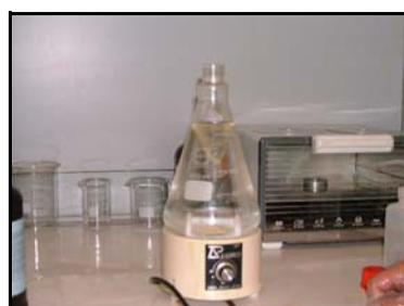
9) Allow the solution in the Erlenmeyer flask to continue stirring for 1 minute.
