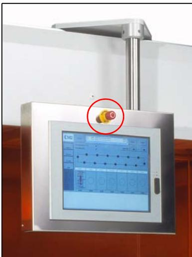
A single Emergency Stop Button is located at the Human Machine Interface. Activating this button results in the immediate stopping of all mechanical movements within the system.
